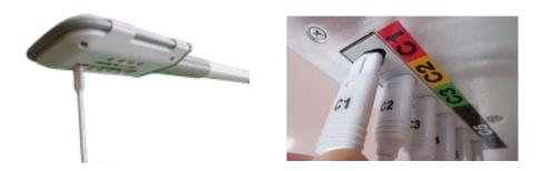
Plug in the vacuum lines into the delta distributor sockets as indicated by the codes.
